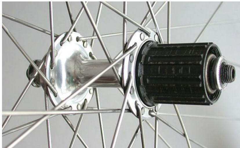
Figure 57 A rear wheel built with option "A" spoking
