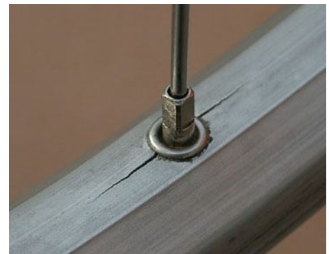
Figure 49 Fatigue crack in rim
